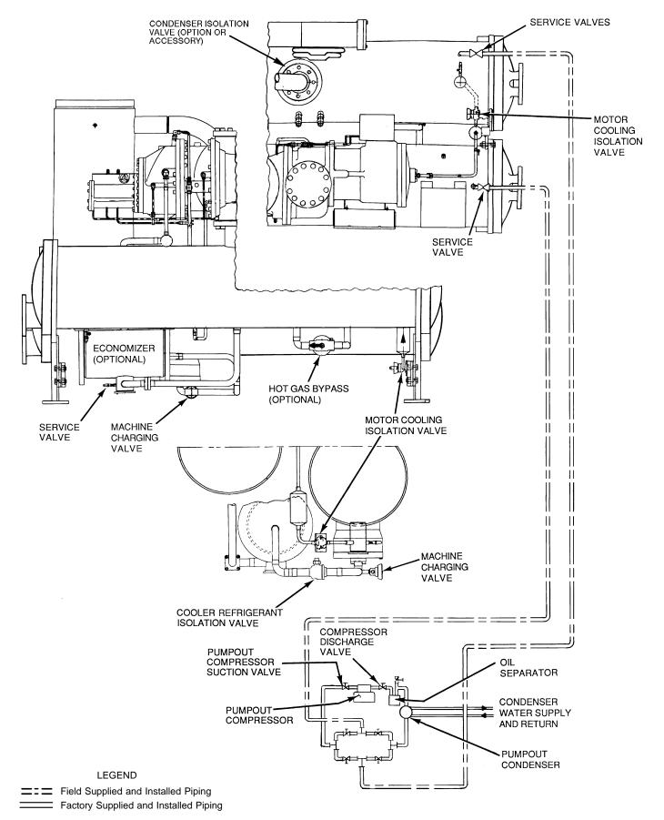
Fig. 24 — Typical Optional Pumpout System Piping Schematic without Storage Tank
